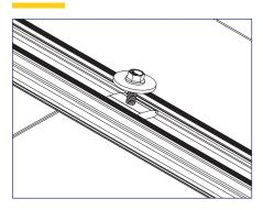
1) Snap the SnapNrack MLPE Rail Attachment Kit channel nut into the desired location on the rail where the microinverter will be installed.
