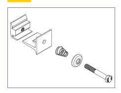
1) Disassemble Ultra Rail Mounting Hardware components, taking note of their installation order and orientation.
