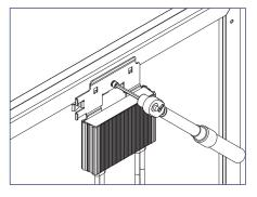
2) Install the optimizer mounting plate onto the module frame and tighten hardware.
