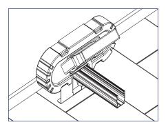
2) Use the reciprocating saw or band saw to cut off the end of the rail (optional).
