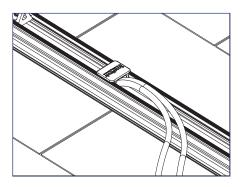
2) Install the Wire Retention Clip by snapping it into place on the rail.
