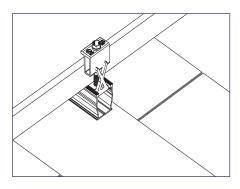
2) Slide the clamp flush to the module with the top lip of the end clamp over the top edge of the module frame.
