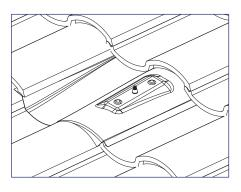
6) Install flashing into place on top of riser, allowing stud to come through hole in Tile Replacement flashing.
