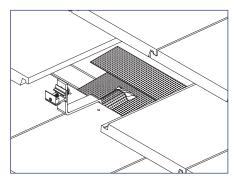
3) If deck level flashing is required, integrate roof felt or a flexible flashing with the existing underlayment and over the Tile Hook.
