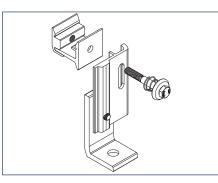
2) Remove bolt from L Foot Extension and install onto preinstalled roof attachment, then set desired height and tighten hardware.
