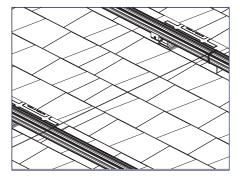
5) Level the remaining rails to the string line by working out from the middle rail, add L Foot Extensions or spacers if needed.
