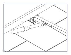
3) Use the pull tab to hold the UEC taut towards the end of the rail and tighten hardware.
