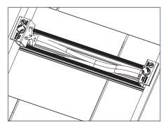
**3)** Place all electrical conductors in the bottom of the rail channel.
