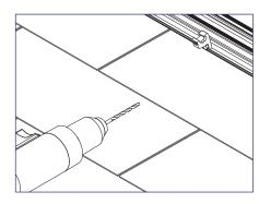
1) Drill and deburr a 1/4" hole in the back side of the rail for the Ilsco lug to attach to, place the bolt through the hole, and attach the lug assembly on **one rail per module row**.
