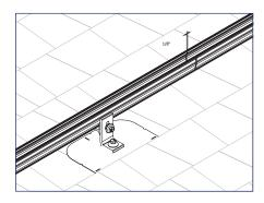
1) Align sections of rail so that ends butt up to each other.
