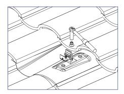
7) Install L Foot onto stud with Umbrella Nut, and tighten hardware.
