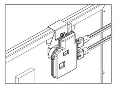
4) Connect the module leads to the microinverter DC connectors.
