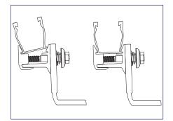
1) Set rails into the attachments by dropping and snapping into the mounts. Connect multiple lengths of rail end to end using the SnapNrack Ultra Rail Splice (see "Ultra Rail Splice" section).
