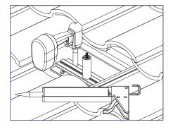
3) Apply roofing sealant and attach the base with (2) 5/16" lag screws, drive lag screws for minimum 2.5" embedment into the roof framing member.
