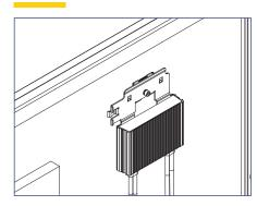
1) Locate the SolarEdge optimizer with Frame-Mounted Module Add-On at a location on the module frame that will not interfere with the SnapNrack rail.
