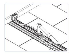
3) Tighten Wire Clamp with 1/2" socket, ensure cables and conductors are aligned in the clamp slots.
