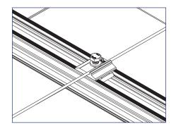
2) Place grounding conductor into slot underneath split ring washer.
