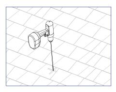
1) Using roof attachment locations drawn during system layout, drill a pilot hole through the roofing material into the roof framing member.
