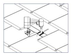
2) Apply roofing sealant and attach the Tile Hook with (2) 5/16" lag screws, drive lag screws for minimum 2.5" embedment into the roof framing member.
