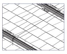
3) Run a string line or spare rail from the bottom rail to the top rail and set desired pitch of the array by adjusting the top rail, add L Foot Extension if needed.
