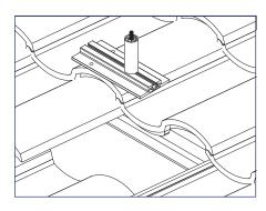
1) Using roof attachment locations drawn during system layout, remove roof tile where the roof attachment will be installed. Slide riser assembly into base channel and snug by hand.
