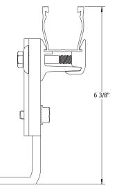
L Foot Extension Provides Up To 3" of Height Adjustment
