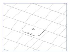
3) Pry up shingles with a breaker bar and install flashing underneath shingle course above pilot hole and, position flashing so cone is in line with pilot hole.
