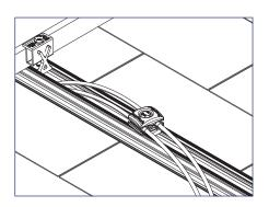
2) With Wire Clamp loose, place conductors or cables in slots.
