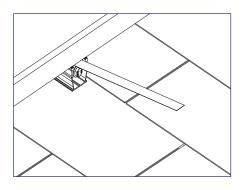
2) Lift the module and slide the clamp far enough under the module to pass the lip of the bottom edge of the module frame.
