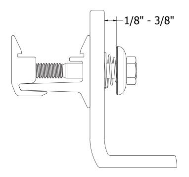
**Recommended Ultra Rail Mounting Hardware Installation**
