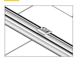
1) Snap the SnapNrack Ground Lug into the rail channel on **one rail per module row**.
