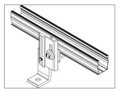
3) Re-install Ultra Rail Mounting Hardware components onto L Foot Extension in the following order:
