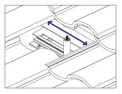
5) Align the riser with the hole in the flashing and tighten riser.
