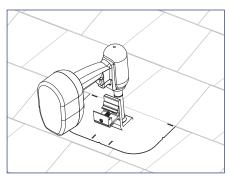
4) Insert Umbrella Lag Screw through Umbrella L Foot and cone in flashing, then drive lag screw for minimum 2.5" embedment into the roof framing member.
