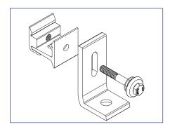
1) Remove Ultra Mount components from roof attachment, taking note of their installation order and orientation.
