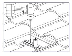
2) Locate base over rafter using riser position and Diagram 1 with measurements found in Table 1, then drill two pilot holes through the roofing material into the roof framing member.
