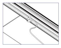
2) Place grounding conductor into slot.
