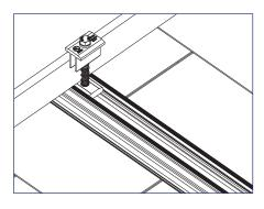
2) Slide the clamp flush to the module with the top lip of the mid clamp over the top edge of the module frame.
