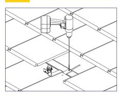
1) Using roof attachment locations drawn during system layout, remove roof tile where the roof attachment will be installed and drill two pilot holes through the roofing material into the roof framing member.
