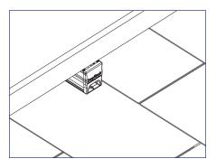
4) Insert SnapNrack Ultra Rail End Cap into the cut end of the rail to create a flush finish to the array.
