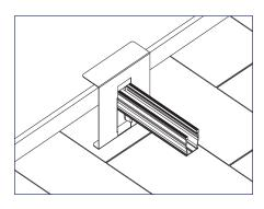
1) Slide the Rail Cutting Tool over the end of the rail and place it so that the upper lip is safely covering the edge of the module (*optional*).
