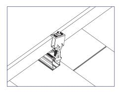
1) Snap the channel nut into the top channel of the rail.
