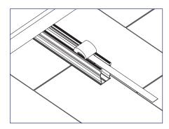
1) Slide the preassembled Universal End Clamp (UEC) into the end of the rail.
