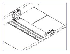
4) Snap Rail Cover into place, enclosing all conductors inside of rail channel.
