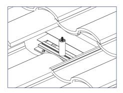
4) If deck level flashing is required, install flexible flashing per the Deck Level Flashing for Tile Replacement Installation Manual.
